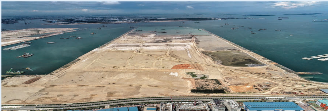
▲ Sustainability is integral to the construction of Tuas Port. More than 50% of the fill materials for Tuas Port Phase 1 reclamation were either dredged from the creation of port's fairways or excavated from other construction projects on land.
