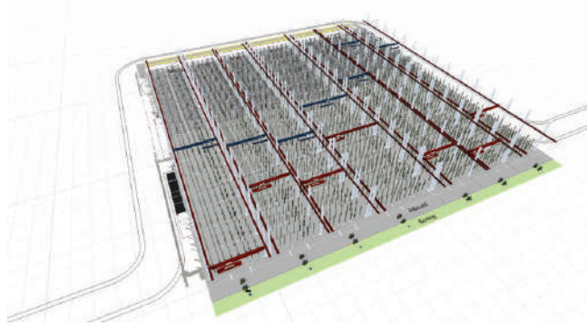
▲ An artist impression of Jurong Port's centralised inventory yard for steel storage which will utilise electric overhead gantry cranes in place of diesel-powered forklifts for the handling of steel cargo.
