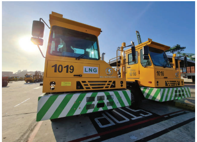
▲ A pilot project for LNG-powered prime movers at PPT.
